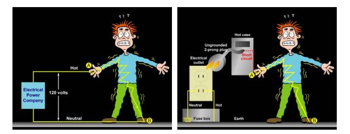
Note, however, that if a 3-pronged plug is employed so that the case is grounded, any short circuit current from a frayed wire or the like will safely return any current to the ground instead of travelling through the victim. This is illustrated below.
