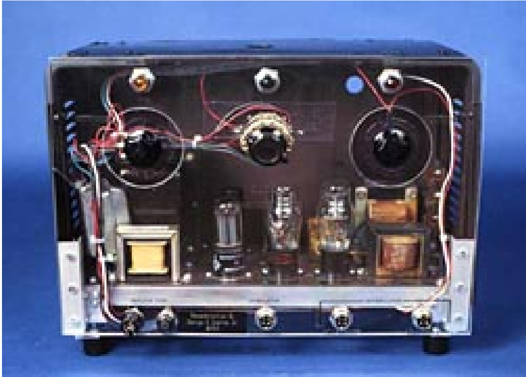
Figure 4: Reproduction of the original Hopps pacemaker. The front panel is of clear plastic to allow visualization of the circuit components.
