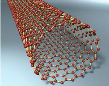
In the case of nanotubes, their special molecular structure results in particularly useful physical properties, such as high tensile strength and excellent electrical and heat conductivity. (Of interest, the chemical bonding of nanotubes is composed entirely of  $sp^2$  bonds, similar to those of graphite. These bonds provide nanotubes with their unusual tensile strength.)
